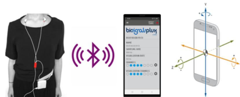
Simultaneous registration of EDA and motion through Wearable Sensors and Smartphone Accelerometer
